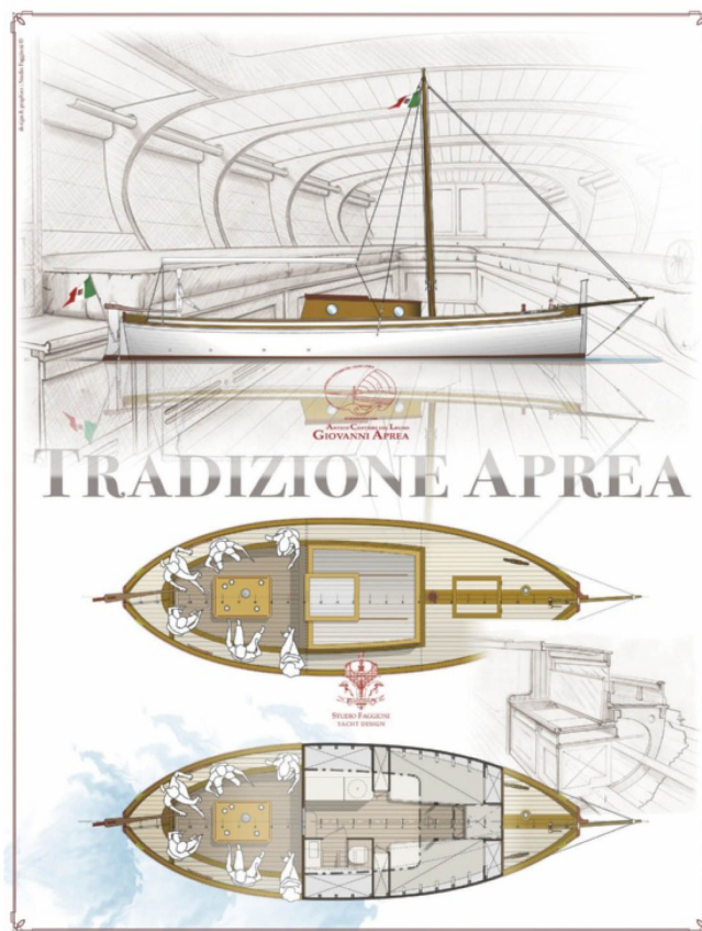
Fig. 1: Gozzo 10, profile with mast for canopy, deck and interior layout. (Studio Faggioni archive).
