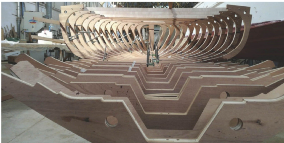
Fig. 2: Framework, in the foreground the floors in marine ply. (Studio Faggioni archive).
