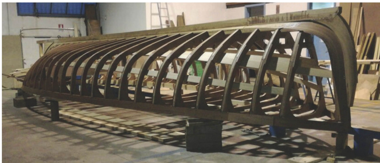
Fig. 8: The hull was overturned to lay on the planking. (Studio Faggioni archive).
